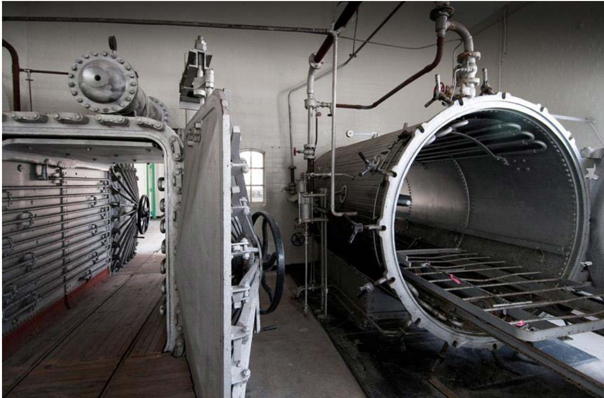
Pictured above: The Boiler House, within the Disinfecting Complex, was built at the Quarantine Station in 1900. It was used to disinfect the luggage and burn contaminated clothes of passengers arriving in Victoria by boat.
